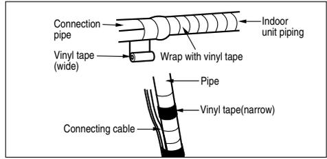
3. Bundle the piping and drain hose together by wrapping them with cloth tape over the range within which they fit into the rear piping housing section.
