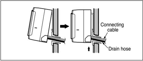
Press the lower left and right sides of the unit against the installation plate until the hooks engage into their slots(clicking sound).
