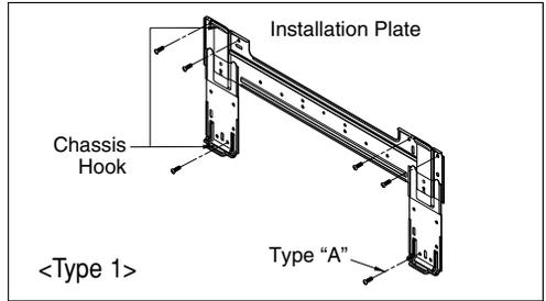
2. Measure the wall and mark the centerline. It is also important to use caution concerning the location of the installation plate—routing of the wiring to power outlets is through the walls typically. Drilling the hole through the wall for piping connections must be done safely.
