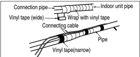
3. Bundle the piping and drain hose together by wrapping them with vinyl tape for enough to cover where they fit into the rear piping housing section.
