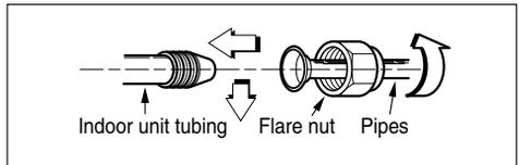
2. Tighten the flare nut with a wrench.
