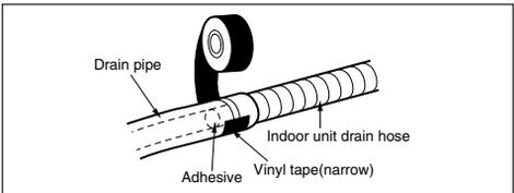
**Wrap the insulation material around the connecting portion.**
