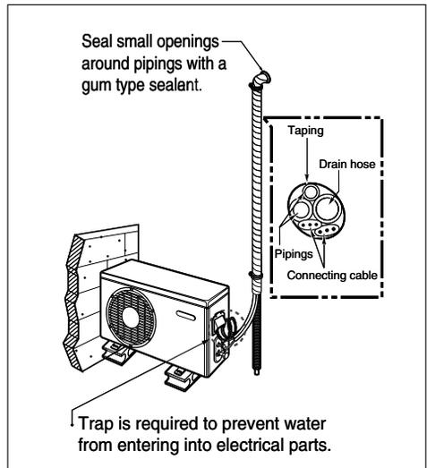
**In cases where the Outdoor unit is installed above the Indoor unit perform the following.**
